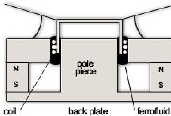
Figure 2: Ferrofluid in audio speaker [6]
